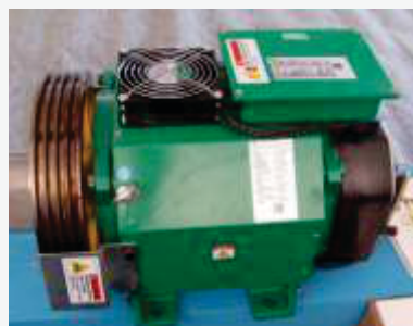
MRL Homme Lift Gearless Machine Capacity 03 to 06 Passengers.
