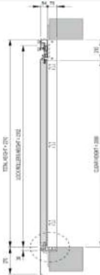
2 Panel Centre Opening Car Door Mechanism
